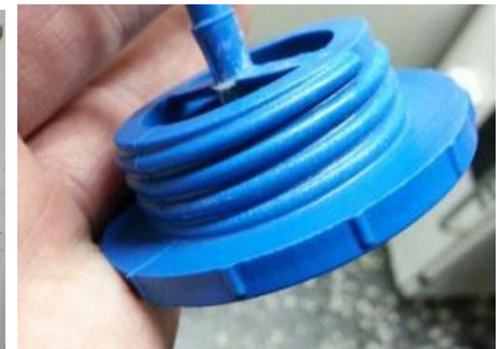
Threaded cap from mold. 20% GF PA 6/6
