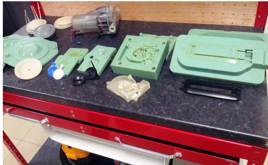
PolyJet molds produce intricate details.
