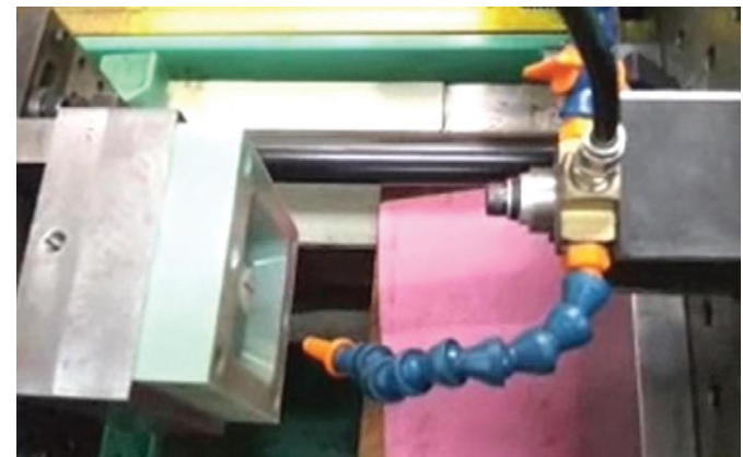
Compressed air cools the core and cavity between cycles.
