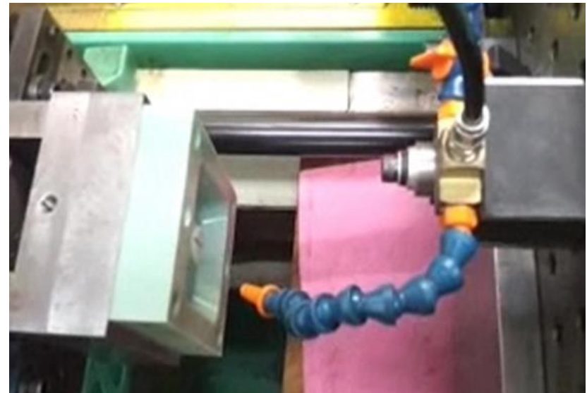
Compressed air cools mold to 50 °C (120 °F).
