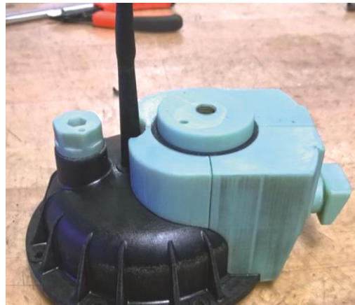
Side view of part with mold and sprue
