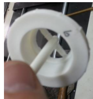
Threaded cap from mold. 20% GF PP
