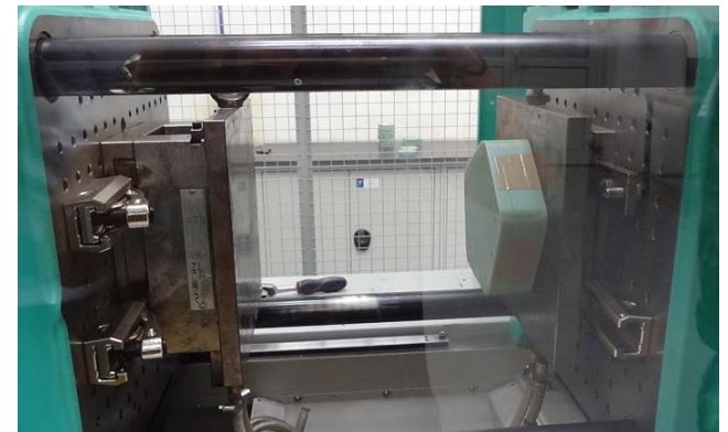
PolyJet molds mounted on steel plates.
